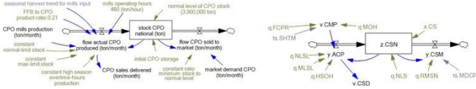
Figure 5. Submodel #1 for market demand input, decoupling from simulated values of CPO production amount: (upper figure) with full notation, and (lower figure) abbreviated version
