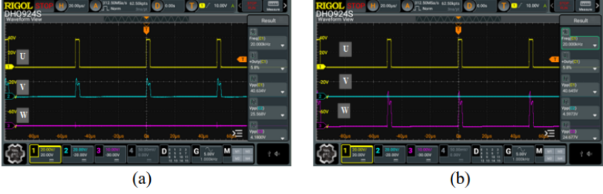
Figure 5. Measured phase voltage waveforms for static Hall states: (a) Hall 100 and (b) Hall 101.
