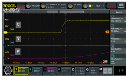
Figure 8. Output waveform at the minimum CW start with 2% duty cycle
