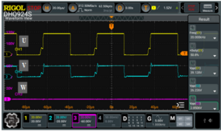
Figure 7. Measured PWM output waveform at 20 kHz switching frequency and 50% duty cycle.
