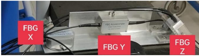
Figure 1. Three-axis Fiber Bragg Grating (FBG) accelerometer
