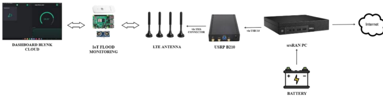
Figure 4. Comprehensive architecture of the portable LTE private system
