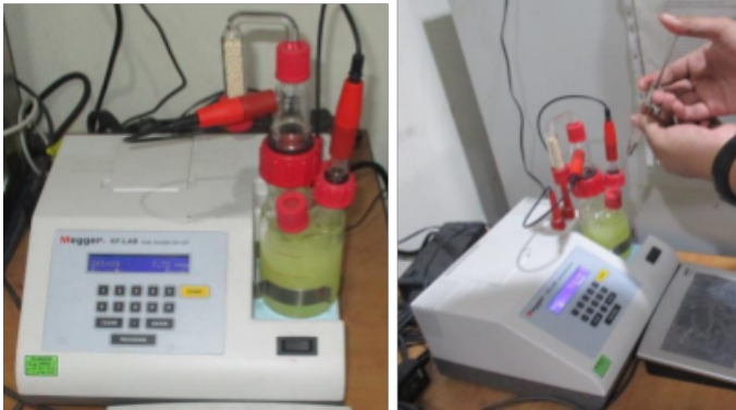
Figure 2. Water content testing on oil using Megger KF-Lab
