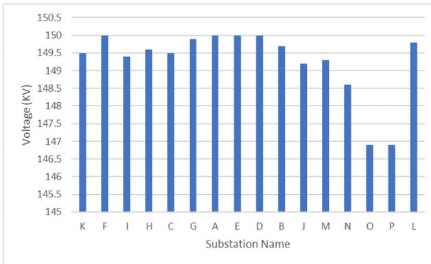
**Figure 6.** Voltage profile of 150 kV busbars in 2024
