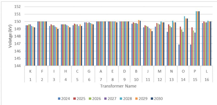
Figure 7. Voltage profile of 150 kV busbars in 2024-2030
