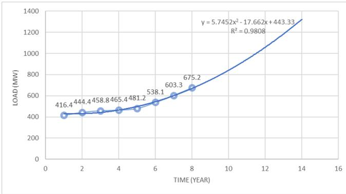
Figure 3. Forecasted peak load curve of the Batam-Bintan power system
