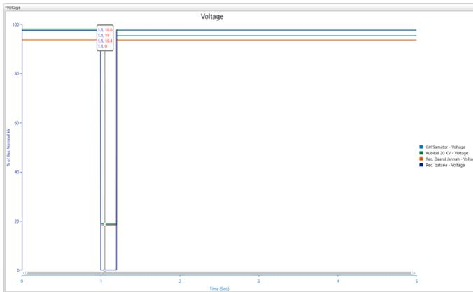
**Figure 18.** Voltage Response to Three-Phase Fault with IS-Limiter Installed at Samator Switching Substation (GH Samator)
