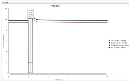
**Figure 12.** Voltage Response to Line 3 Phase Fault with SVC Installed at the 20 kV Incoming Busbar of GI Kenten
