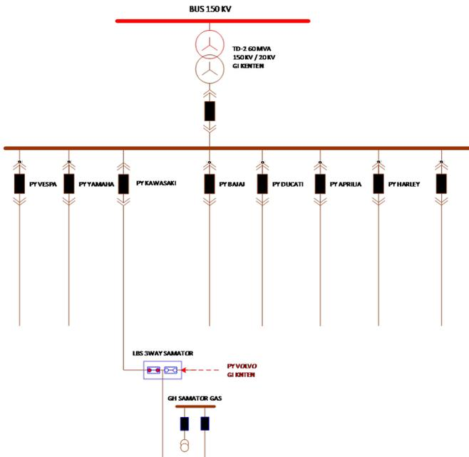
Figure 3. Single Line Diagram of Kenten Main Substation – Distribution Transformer #2
