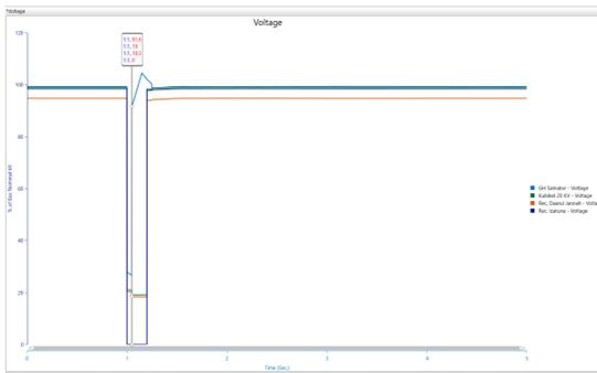
**Figure 20.** Voltage Response to Three-Phase Fault with DRUPS Installed at Samator Switching Substation (GH Samator)
