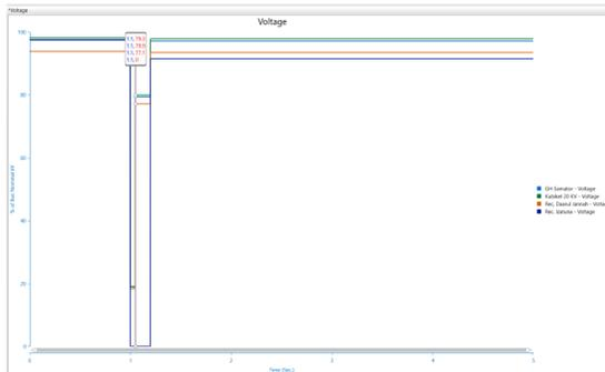
**Figure 16.** Voltage Response to Three-Phase Fault with IS-Limiter Installed at the Outgoing Side of the Fault-Affected Feeder of Kenten Main Substation (GI Kenten)
