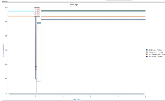
**Figure 15.** Voltage Response to Line-to-Line Fault with IS-Limiter Installed at the Fault-Affected Feeder of Kenten Main Substation (GI Kenten)
