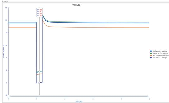
**Figure 11.** Voltage Response to Line-to-Line Fault with SVC Installed at the 20 kV Incoming Busbar of GI Kenten
