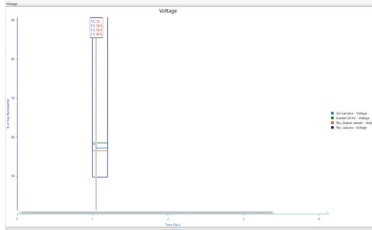
**Figure 17.** Voltage Response to Line-to-Line Fault with IS-Limiter Installed at Samator Switching Substation (GH Samator)
