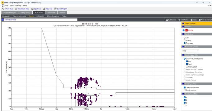
Figure 6. PQM Fluke Event, Distribution Dip & Swell Analysis Based on ITIC Curve Tolerance
