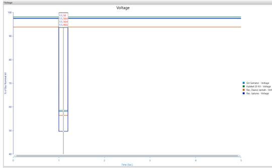
Figure 9. Voltage Response During Line-to-Line Fault Under Normal Operating Conditions
