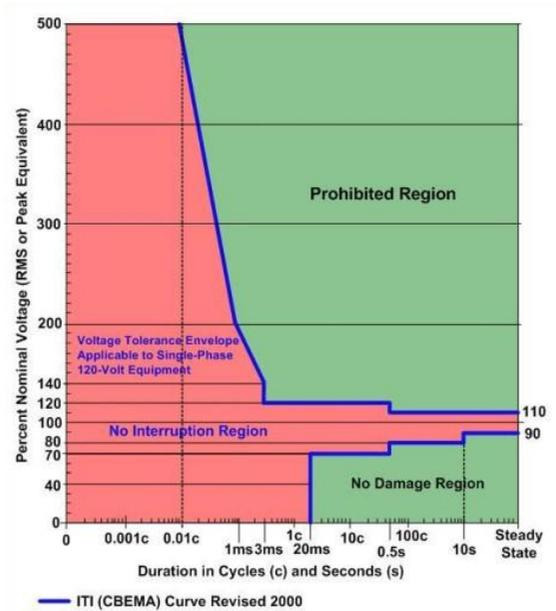
Figure 2. ITIC Curve in Duration of Cycles (c) and Seconds (s)
