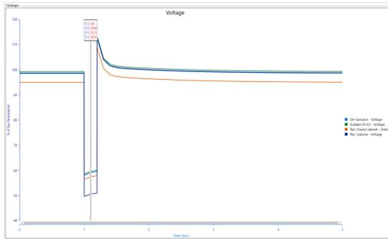
**Figure 13.** Voltage Response to Line-to-Line Fault with SVC Installed at the Fault-Affected Feeder of Kenten Main Substation (GI Kenten)
