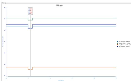
**Figure 8.** Voltage Response During Line-to-Ground Fault Under Normal Operating Conditions
