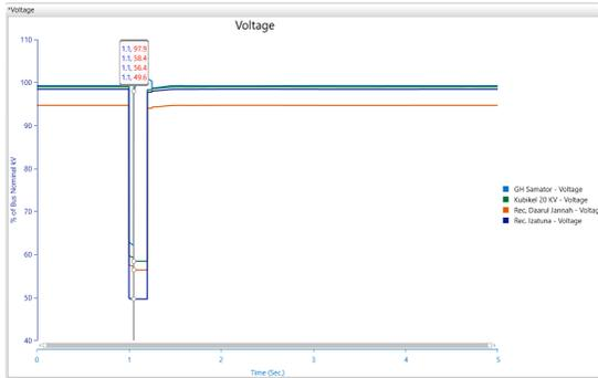
**Figure 19.** Voltage Response to Line-to-Line Fault with DRUPS Installed at Samator Switching Substation (GH Samator)
