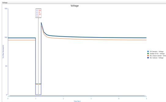
**Figure 14.** Voltage Response to Three-Phase Fault with SVC Installed at the Fault-Affected Feeder of Kenten Main Substation (GI Kenten)
