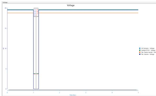
Figure 10. Voltage During Three-Phase Fault Under Normal Operating Conditions
